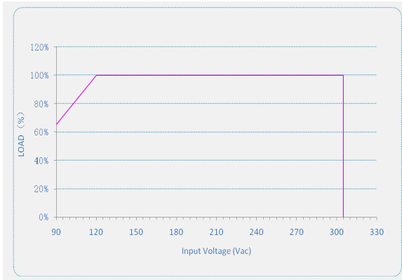
Output Power Vs. Input Voltage
