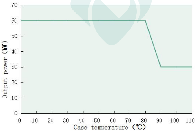
Output power VS Tcase (DL-60H-56A/P-MXC)
